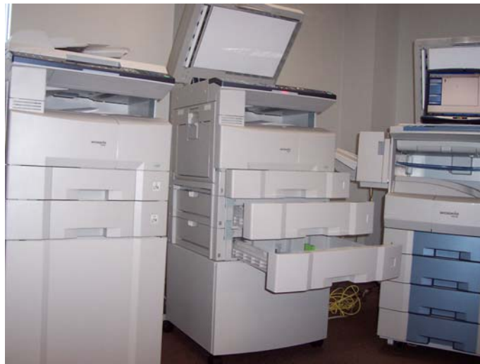
Universal Paper Drawer with Sliding Guide and Pre-Defined Guide slots
